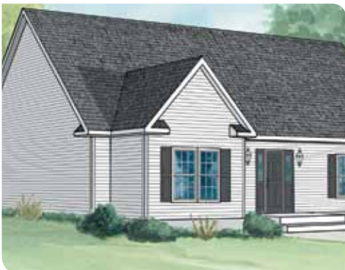
Decorative Shingle Return
